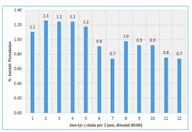
Figure 4a. Customer's 24-hour water usage pattern in Kec. Mijen
