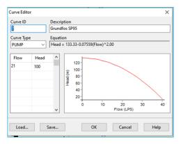
Figure 6. Pump Curve Editor in Epanet
