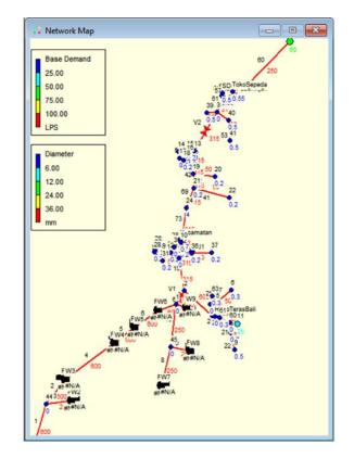
Figure 8. Pump-Pipe Network Model in Kec. Mijen on Epanet
